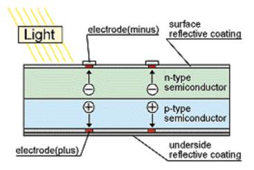
Figure 1: Silicon Solar Cell and its working mechanism (Source: global.kyocera.com)
