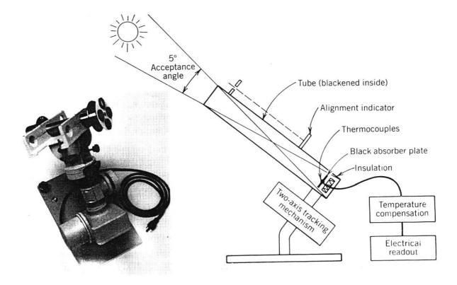
Figure 28: A Normal Incidence Pyrheliometer (NIP) used for measuring the direct component of solar radiation (Source: Eppley Laboratory, Inc.)
