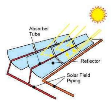
Figure 13: Parabolic Trough (Source www.hkengineer.org.hk)
