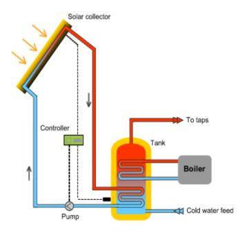
Figure 21: Schematic of Solar Water Heating system
