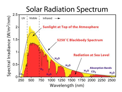
Figure 5: Solar Spectrum (Source: www.juliantrubin.com)
