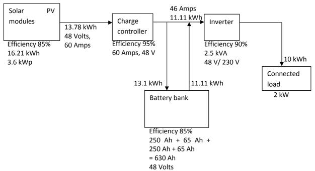
Figure 30: Standalone solar PV power plant design diagram
