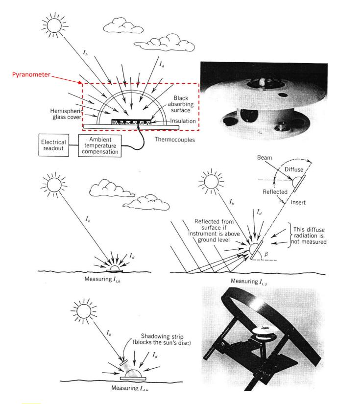
Figure 26: The pyranometer and its use in measuring global horizontal, tilted global, and the diffuse components of solar irradiance (Source: Eppley Laboratory, Inc.)
