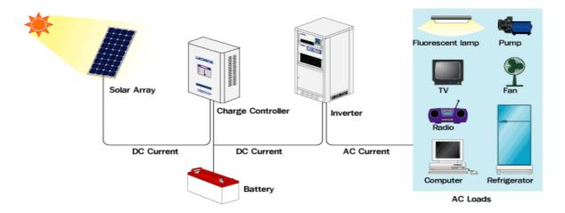
Figure 18: Schematic of Solar Home Lighting System
