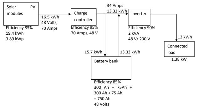
Figure 29: SPV Home Lighting System design diagram
