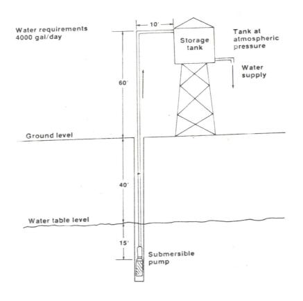
Figure 32: System Sizing of Solar PV Water pump
