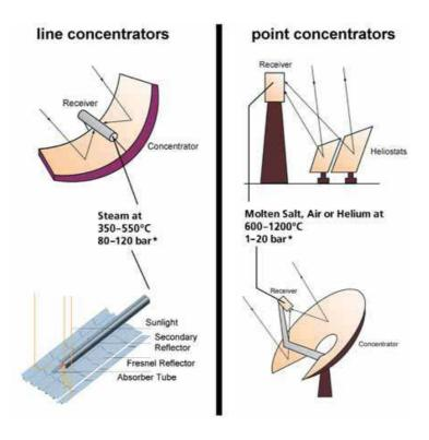
Figure 9: Concentrator arrays (Source)
