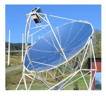
Figure 15: Dish Stirling (Source: intersol.se)
